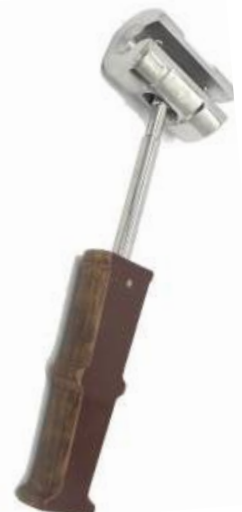
A hammer used by an astronaut during the Apollo moon landings. This hammer has a mass of 1300 g and is 39 cm long with a 16 cm head
